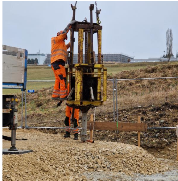
PDA on micropile (StreetBox Vallorbe, VD)
